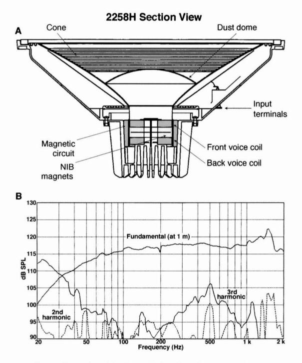
Figure 5. Section view of the JBL 2258H driver (A); fundamental and distortion response at 80 watts (B). (Distortion raised 20 dB)
