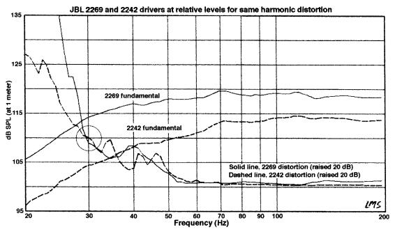
Figure 4. A comparison of output levels of JBL 2242H and 2269H drivers at the same distortion level.
