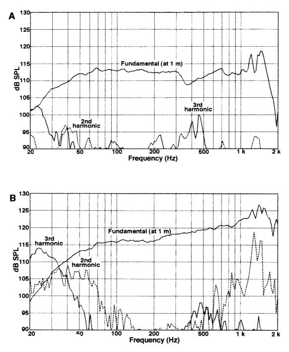
Figure 3. Fundamental and distortion response of 2269H driver at 80 watts (A); fundamental and distortion response of 2242H driver at 80 watts (B). (Distortion raised 20 dB)
